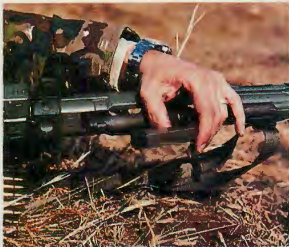
UPPER LEFT: Weapon's rear sight is adjustable to 1,000 meters. ABOVE: MG82 barrels feature hard-chromed bores and chambers, are available with either 1:7-inch or 1:12-inch twist. LEFT: Barrel may be changed within a few seconds. Note carrying handle attached to it.
